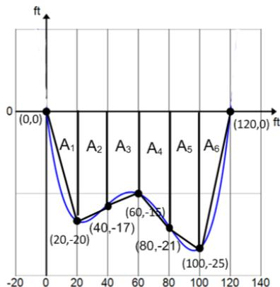
$$\begin{aligned} A &= A_1 + A_2 + A_3 + A_4 + A_5 + A_6 \\ &= 200 \text{ ft}^2 + 370 \text{ ft}^2 + 320 \text{ ft}^2 + 360 \text{ ft}^2 + 460 \text{ ft}^2 + 250 \text{ ft}^2 \\ &= 1,960 \text{ ft}^2 \end{aligned}$$
